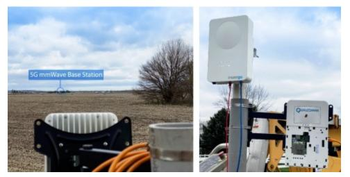
Unprecedented range and sustained speeds - Recent 5G mmWave field tests on the UScellular network demonstrated sustained average downlink speeds of ~1 Gbps and peak speeds over 2 Gbps at a distance of 7 km — the farthest 5G mmWave Fixed Wireless Access (FWA) connection in theU.S. This milestone was achieved using Ericsson infrastructure and an Inseego Wavemaker fixed wireless outdoor gateway, powered by the Qualcomm 5G Fixed Wireless Access Platform gen 1. (Photo: Business Wire)
